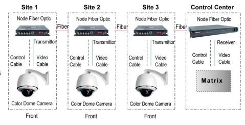
network video encoders working with the on-site digital video storage server, and, ultimately, transmitted to the monitoring and management center via the fiber ring network. As a result, authorization levels can be created that allow the center to call up, control and store video from the edge sites remotely. Video also can be called up and transmitted manually, by schedule, or triggered by events.
