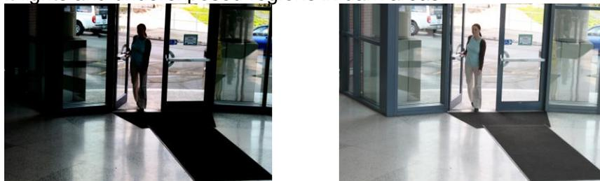
Contrarily, an all-digital technology can provide Wide Dynamic Range (WDR) in which each of the hundreds of thousands of pixels acts like an individual, self-adjusting camera. Wide Dynamic Range (WDR) is the ratio of the brightest pixel that can be captured by the imaging system to the darkest pixel that can be captured. With high resolution cameras especially, users need a WDR of 17 bits, > 100db.
